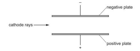
The cathode rays are deflected as they pass between the plates.
